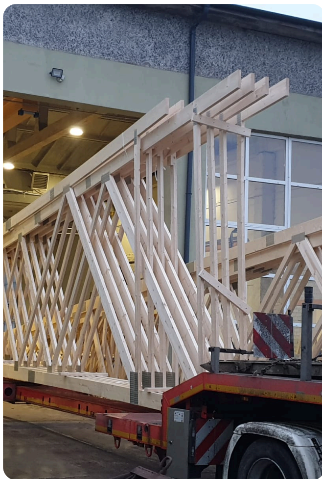
Roof truss leaving the factory
