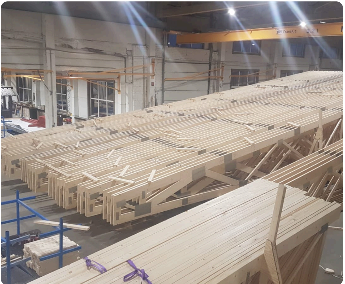
Roof trusses stacked in the factory hall.
